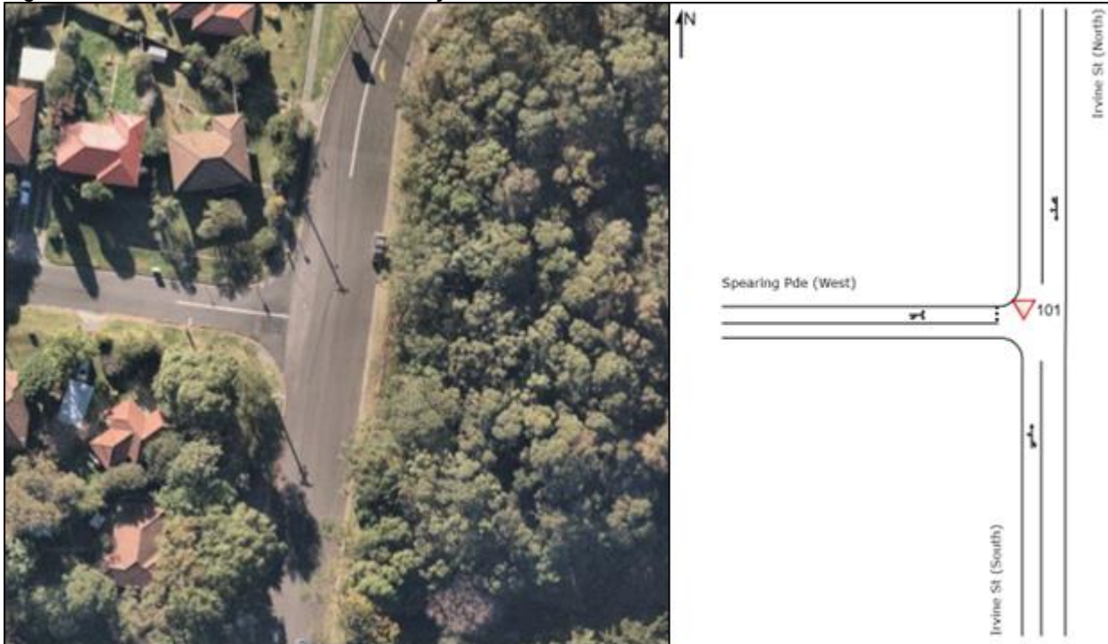
Figure 4-11: Intersection 5 – SIDRA Layout
