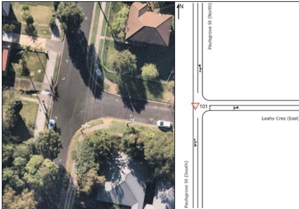
Figure 4-14: Intersection 8 – SIDRA Layout
