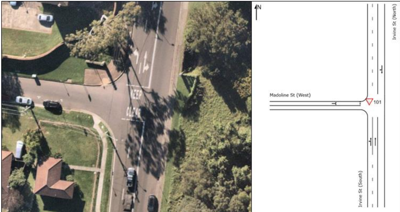
Figure 4-8: Intersection 2 – SIDRA Layout
