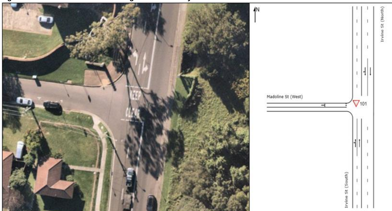
Figure 4-20: Intersection 2 – Mitigation SIDRA Layout
